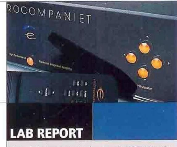
Though beaten over certain parameters by others in this strong test group, this amp presented generally convincing measurements overall. The power supply measures very well, producing a maximum output of 22A into our stress-testing jig, with voltage clipping taking place at 23V (8-ohm simulated load).
