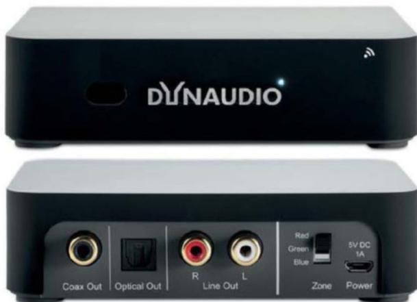
● The Xeo Link receives wireless signals from the Xeo Hub and also outputs analog and digital signals.
