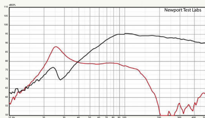
Figure 3. Low frequency response of front-firing bass reflex port (red trace) and woofer. Nearfield acquisition. Port/woofer levels not compensated for differences in radiating areas. [Dynaudio Emit M30 Loudspeaker]
